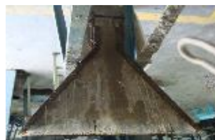
Plate 7: Photograph of V-Funnel Test on SCC
