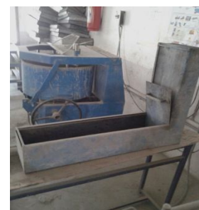
Plate 9: Photograph of L-Box Test on SCC
