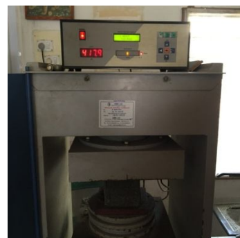
Plate 14: Photograph of Specimen during Compression
