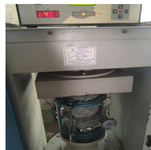
Plate 16: Photograph of Testing of Elastic Modulus by using Extensometer
