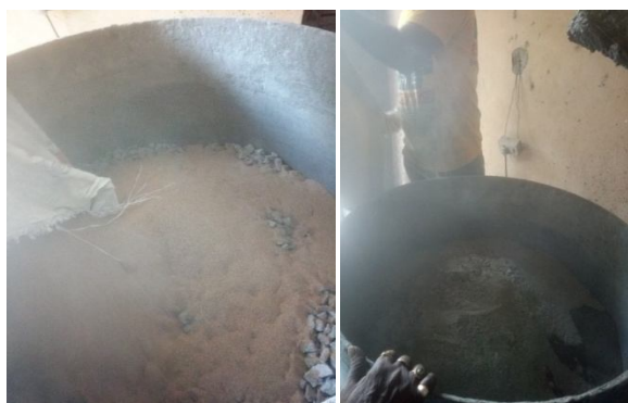
Plate5: Photograph of dry constituents of SCC with River sand
