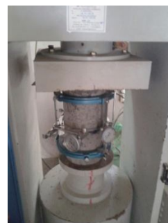
Plate 17: Photograph of Setting of Extensometer
