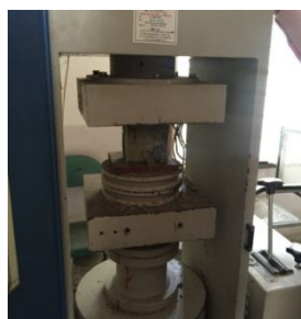
Plate 13: Photograph of Loading Unit of CTM
