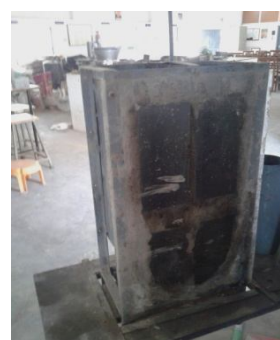
Plate 8: Photograph of U-Box Test on SCC
