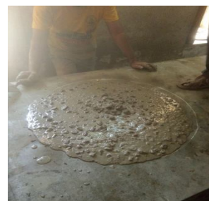
Plate 6: Photograph of Slump Cone Test
