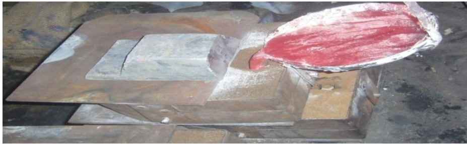
Figure 3.11: Molten material pouring (temperature 650°C)
