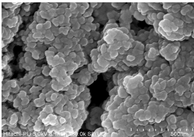
Figure 8: FESEM image of iron oxide NPs prepared using FLE.
