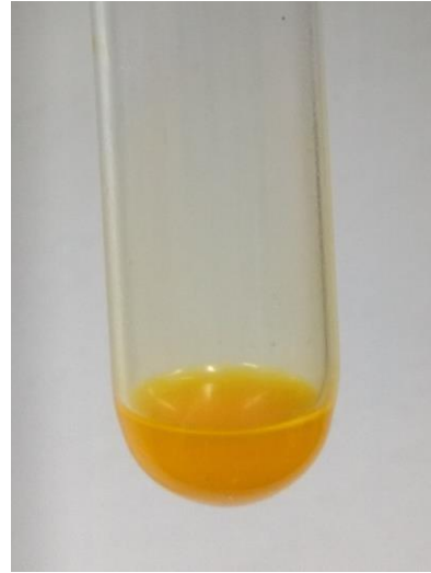
Fig.6 Absence of lead in Shankha Bhasma (Sample3)
