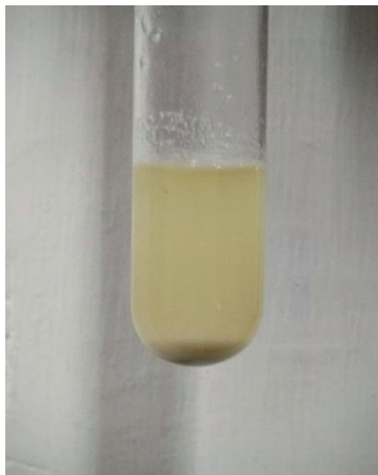
Fig.3 Presence of lead in Vanga Bhasma Bhasma (Sample2)
