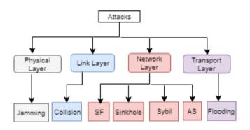
Acknowledgment spoofing (AS) - In this attack generally, the attacking node sends false or fake information to its neighbour nodes. For instance, claiming that sensor node is deceased when it is actually active. The type of this attack is called as Acknowledgement Spoofing.
