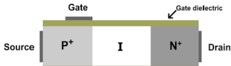
Fig.1. Structure of TFET Device
