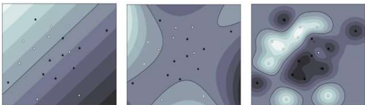
(a) Linear kernel. (b) Polynomial kernel. (c) Radial Basis Function (RBF) kernel.
