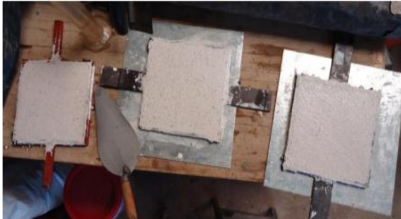
Figure: Making the tiles with the moulds
