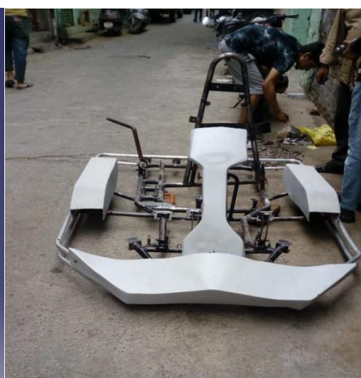
Figure 2: Bodyworks position on frame
