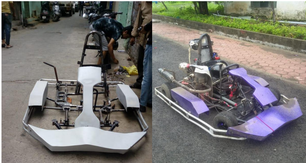
Figure 3: Bodyworks after surface finishing on chassis Figure 4: Bodyworks after painting
