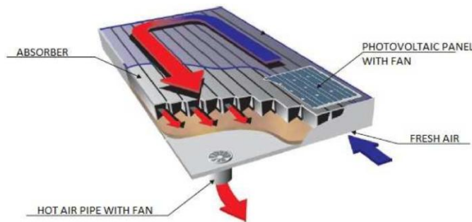
Fig 9: Solar Air Collector of Twin and Top[7]
