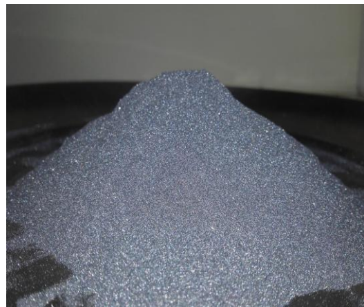
Figure 4. Powder Boron Carbide 200 \mu\text{m}
