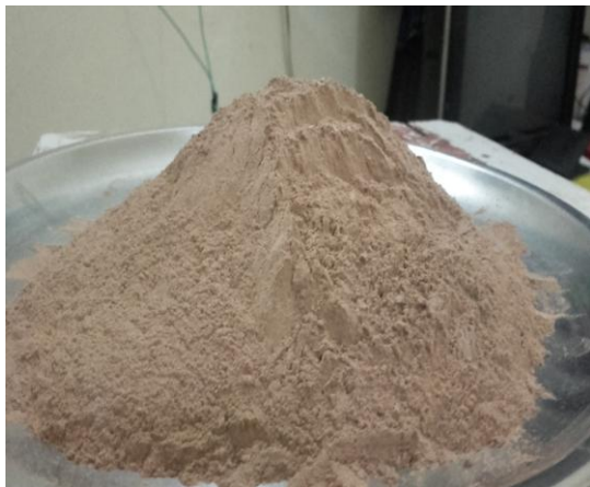
Figure 3. Powder Kyanite 74 \mu\text{m}
