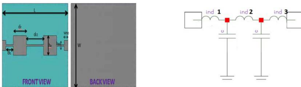
Fig. 1. Micro strip low pass filter and its equivalent circuit
