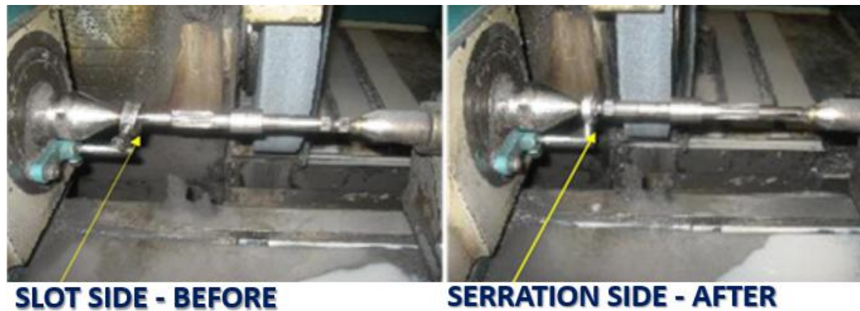
Figure 3. Clamping moved to serration side before and after VSM implementation
