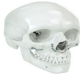
Figure 7 - Human skull developed by RP technique[2]
