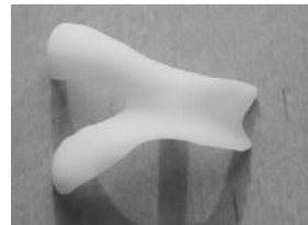
Figure11(c)- RP pattern of Hemi-Knee joint
