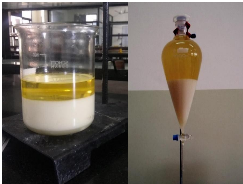
Fig. 3 Glycerol separation from Biodiesel
