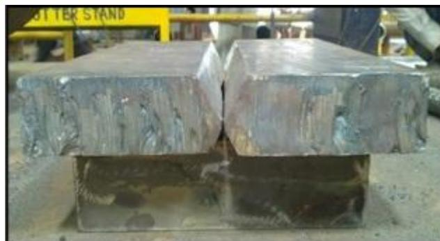
Figure 1: Double V-Butt joint in specimen
