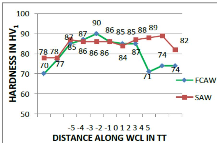
Figure 11 Hardness Testing results along T-T
