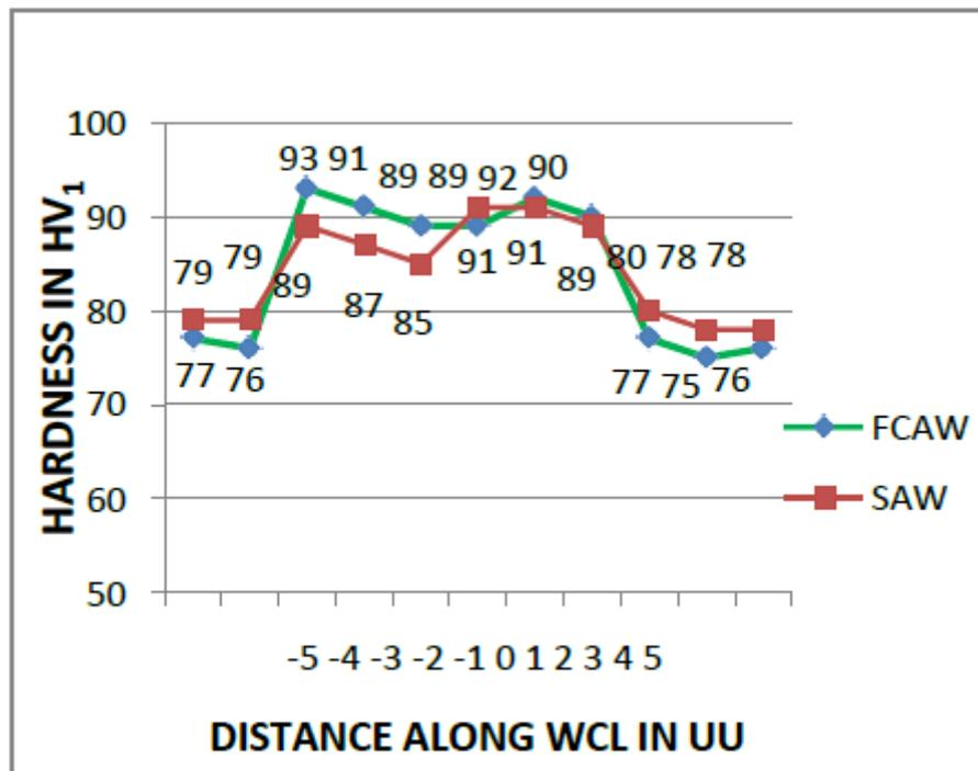
Figure 10 Hardness Testing results along U-U
