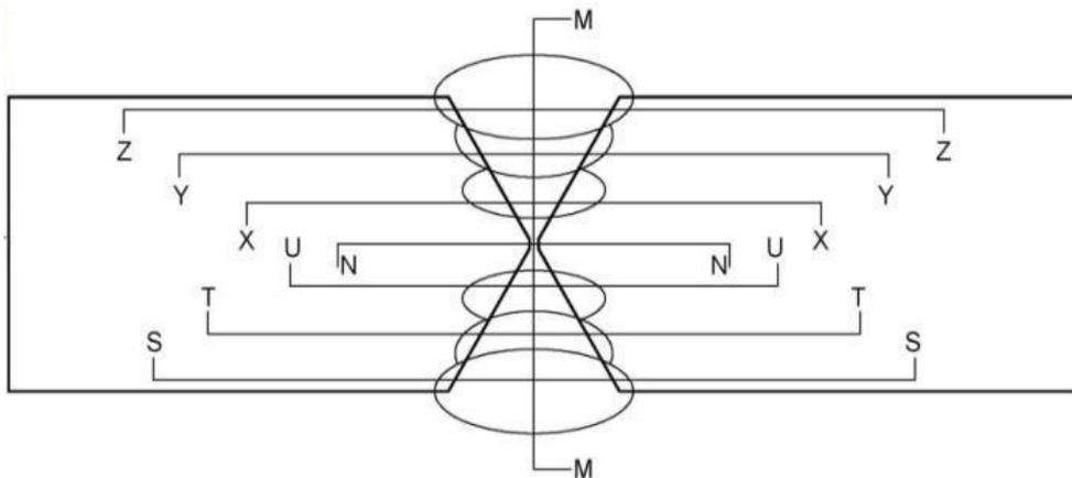
Figure 4 Hardness Testing Locations at different axis
