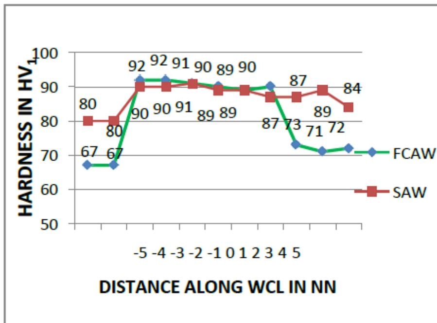
Figure 9 Hardness Testing results along N-N
