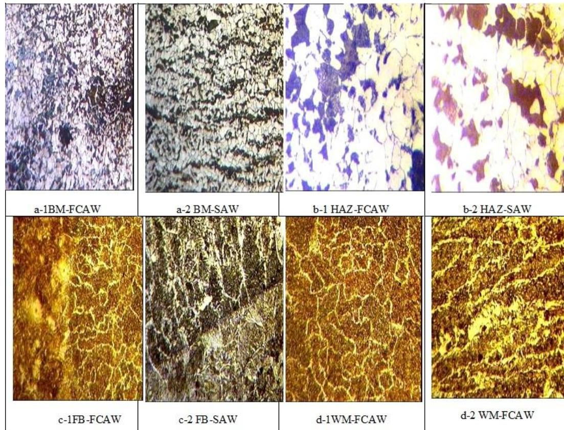
Figure 3: Different Microstructure of FCAW and SAW welding at different zones (a-1) Base metal at 100X of FCAW test specimen (a-2) Base metal at 100X of SAW test specimen (b-1) HAZ at 100X of FCAW test specimen (b-2) HAZ at 100X of SAW test specimen (c-1) FB at 100X of FCAW test specimen (c-2) FB at 100X of SAW test specimen (d-1) WM at 100X of FCAW test specimen (d-2) WM at 100X of FCAW test specimen.
