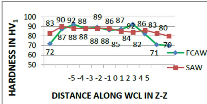
Figure6 Hardness Testing results along Z-Z
