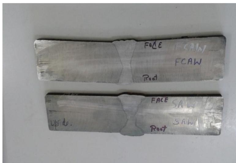
Figure 2 Macro Examinations of FCAW and SAW
