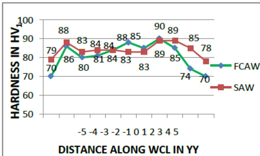
Figure 7 Hardness Testing results along Y-Y
