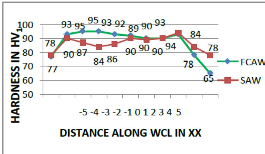
Figure 8 Hardness Testing results along X-X
