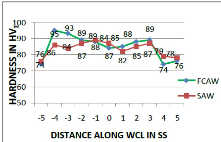
Figure 12 Hardness Testing results along S-S
