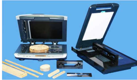
Fig 3 Scanners utilized in WinDENDRO for tree ring analysis [18]
