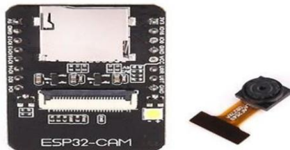
Figure 4 ESP- 32 module and its Camera
