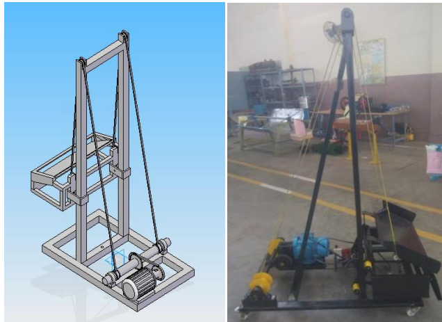
Figure.6.1.a & b Semi-automated wall plastering machine.
