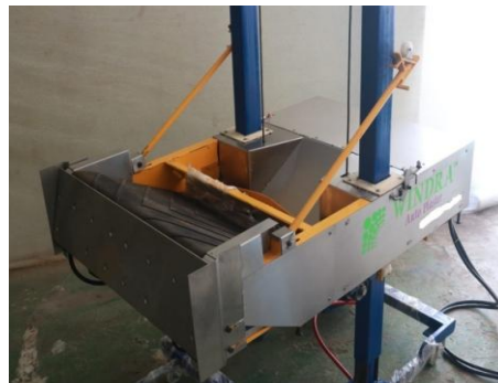
Figure.3.2 Automated method of plastering machine.
