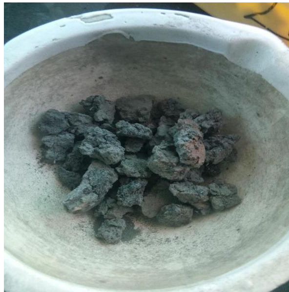
Fig 2: Grinding of dried sewage sludge collected from phagwara drain passing Lovely Professional University.
