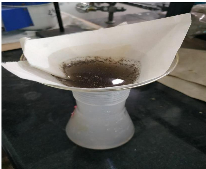
Fig 8: Filtration of solution containing Adsorbent and cd solution after batch process
