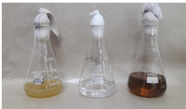
Fig 2: (a) leaf extract, (b) AgNO 3 solution and (c) E. globulus synthesized silver nanoparticles
