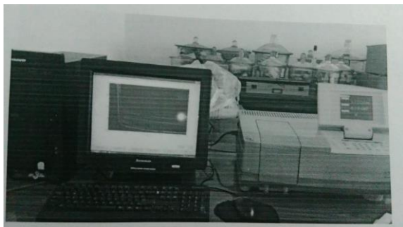
Fig.1 UV Spectrometer used for recording spectrographs.
