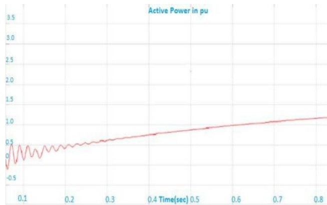
Fig. 9 Controller output for K_{P1} = 0.06 and K_{I1} = 1
