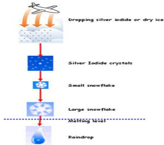
Figure 17 Effect Of Dispersing Silver Iodide Or Dry Ice Particles(Source-Centre For Earth Atmosphere And weather Modification Technologies, JNTU, Hyderabad)
