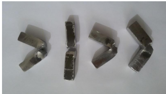
Figure 1.1: Specimens after impact test
