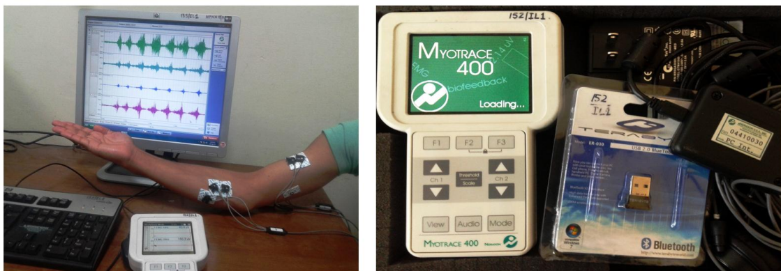
Fig. 2. Complete EMG signals acquisition setup with myotace 400 device
