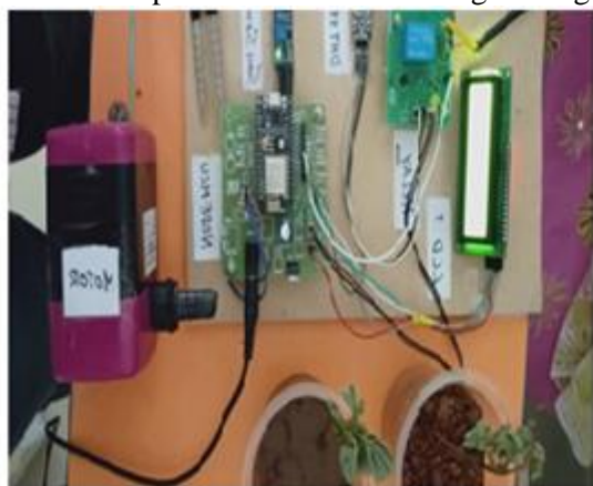
Fig.1: low cost smart irrigation using MQTT protocol
