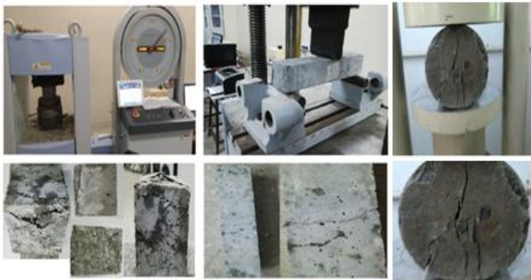
Fig. I Different Testing and Crack Propagation
