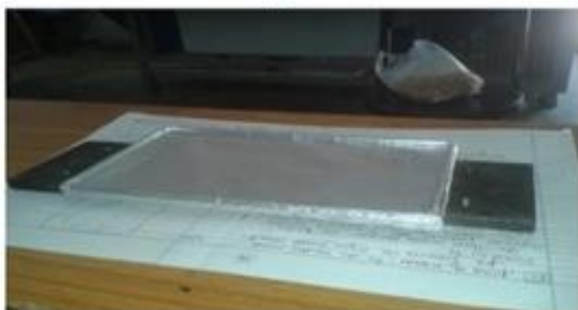
Fig. 2 aluminum wrapped mould cavity
